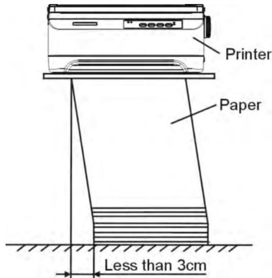
3. Front and back positioning: The distance between the rear of printer and the wall should be more than 60 cm. To avoid paper jam, the distance between the continuous paper and the edge of desk should be 10~15 cm.
