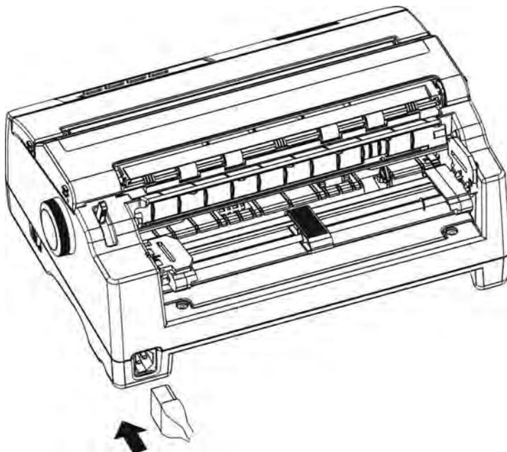
Connect the power cord to the power inlet of the printer. Connect the power cord plug to a mains socket. Switch on the printer.
