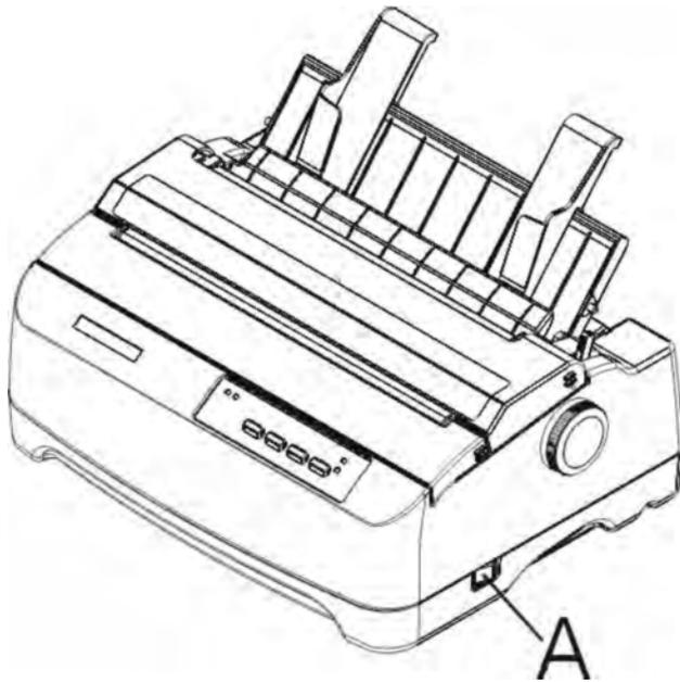
Make sure that the power switch "A", located to the right side of the printer, is in the "O" (off) position.
