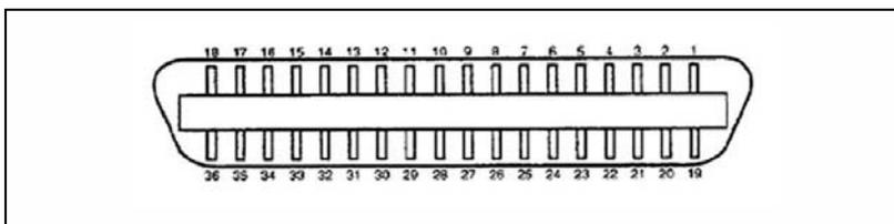
Note: Any external devices connected to the parallel port should not draw current exceeding 200 mA from pin 18; otherwise it may affect the printer operation.
